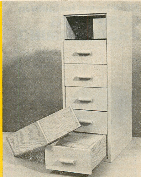
Small cabinet is open at rear; larger size will need a back to reinforce frame.
