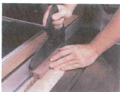
Figure 1: After cutting stock to size for the upper cab, adjust your blade height and fence and make two cuts to define the inside edges of the posts.
