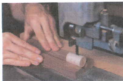
Figure 6: Cut a V-groove in scrapwood and hot glue the barrel into the groove. The hot glue will hold the barrel steady while you bandsaw it in half.
