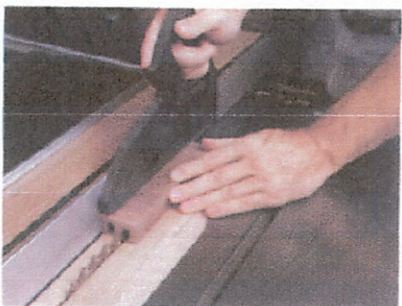
Figure 2: Continue adjusting the fence about 1/16" at a time to make a series of passes for nibbling away the waste in the cab.
