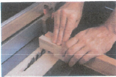
Figure 4: Use a 1/2" dado blade to cut notches for the rear wheels in the truck base. Make several passes, and use a set-up block to limit the cuts.
